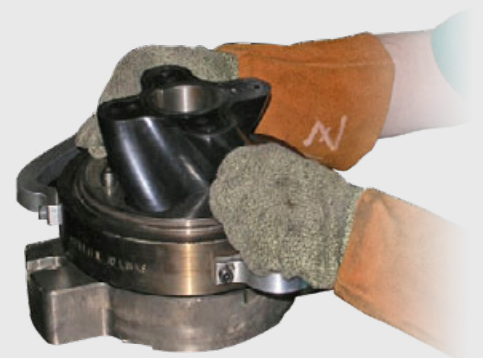
Vulcanisation – a key process in the production of elastomeric rotors
