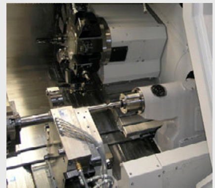
High precision, repeatable production on 7 axis CNC machines (drive shaft shown)
