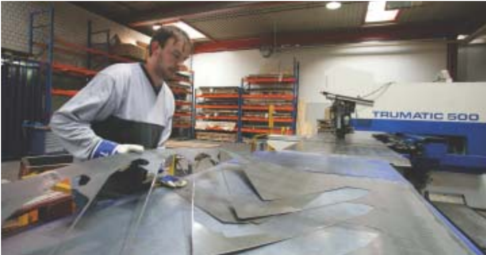
Precision: Quality knows no compromises at the Meppen factory. The picture shows the sheet metal processing centre in the fabrication area.
