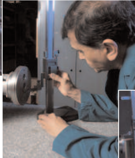
Technicians measuring the dimensions of pump components with precision calipers: Liquiflo pump components are precisely manufactured to tolerances as low as .0004 inches (10 microns).
