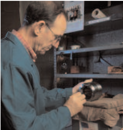
Technician assembling an outer magnet for a mag-drive pump: Liquiflo produces a variety of magnetic couplings to fit each pump model and match the torque transmission required by the application.
