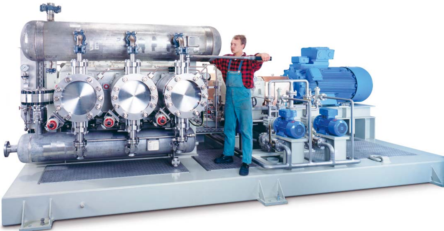
Example chemistry: highly corrosive intermediate products 14 m 3 /h, 350 bar, G3R, M500
