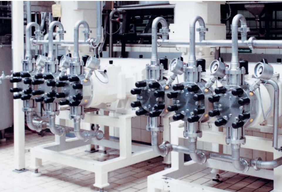
Example food production: gentle conveying of food-stuffs, 2x G3S, M500, 6 m 3 /h at 90 bar
