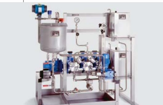
Precise and reproducible: fully automatic compact package for recipe controlled production of dispersion adhesives
