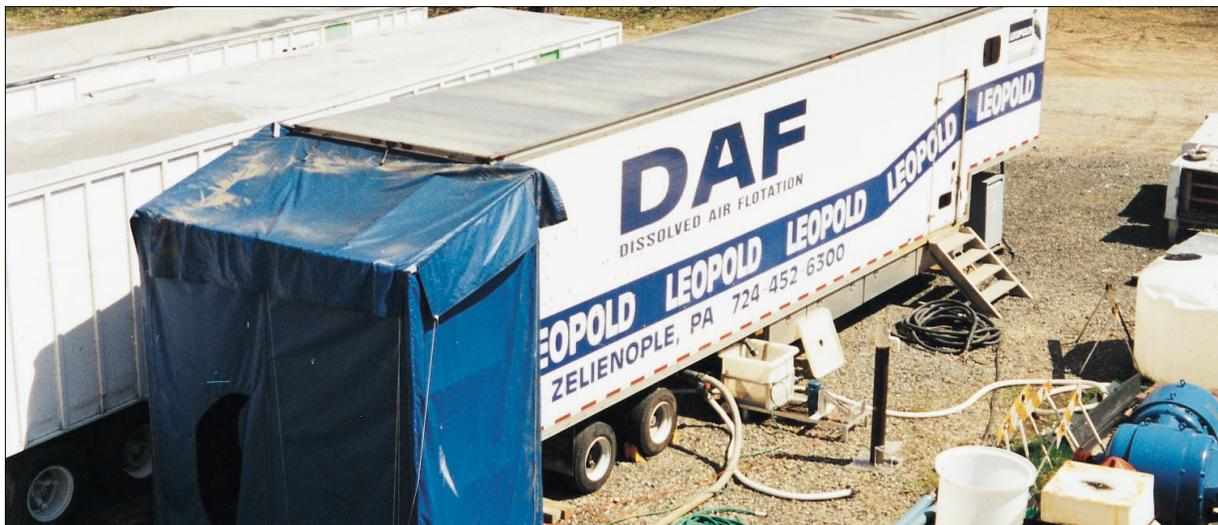
The Leopold mobile Clari-DAF system pilot plant gathers data every five minutes around the clock for weeks under actual operating conditions to determine the most appropriate flocculation conditions for designing and engineering a full-scale Clari-DAF system installation.
