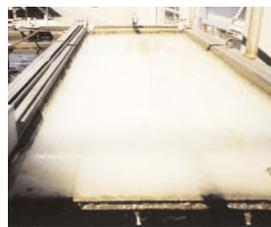
The Clari-DAF system creates a milky solution of hundreds of millions of microbubbles 20 to 100 microns in size that rapidly float suspended particles to the surface for removal.
