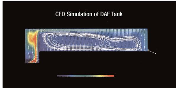
Computer modeling allows Leopold to optimize each Clari-DAF system installation to each plant's particular needs and operating conditions.
