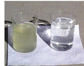
Shortly after start-up, the Leopold Clari-DAF system can produce crystal clear water.
