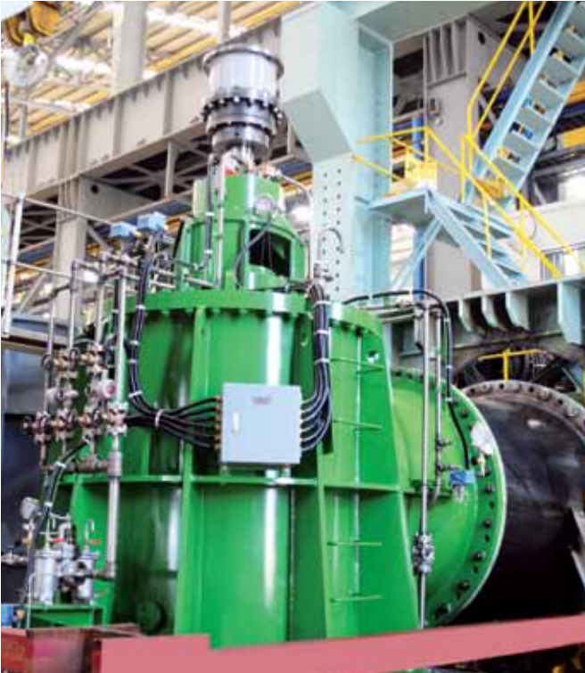
Shop test of Kudankulam Nuclear Power Plant, INDIA Sea Water Pump (735.5m 3 /min X 15.9m X 3200kW, Model 2200VKAM)
