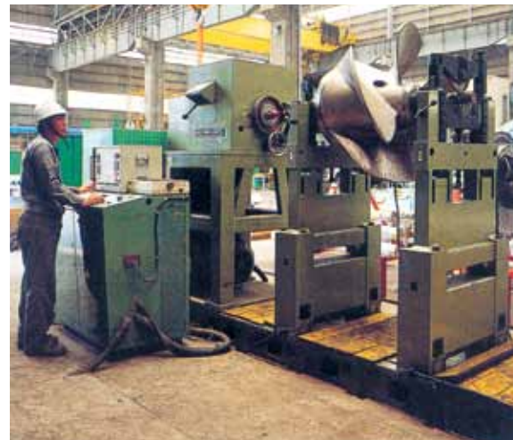
Computer aided dynamic balance test of impeller
