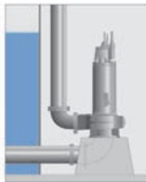
**NT** – A vertical, dry-pit or in-line installation with flange connections for suction and discharge piping.
