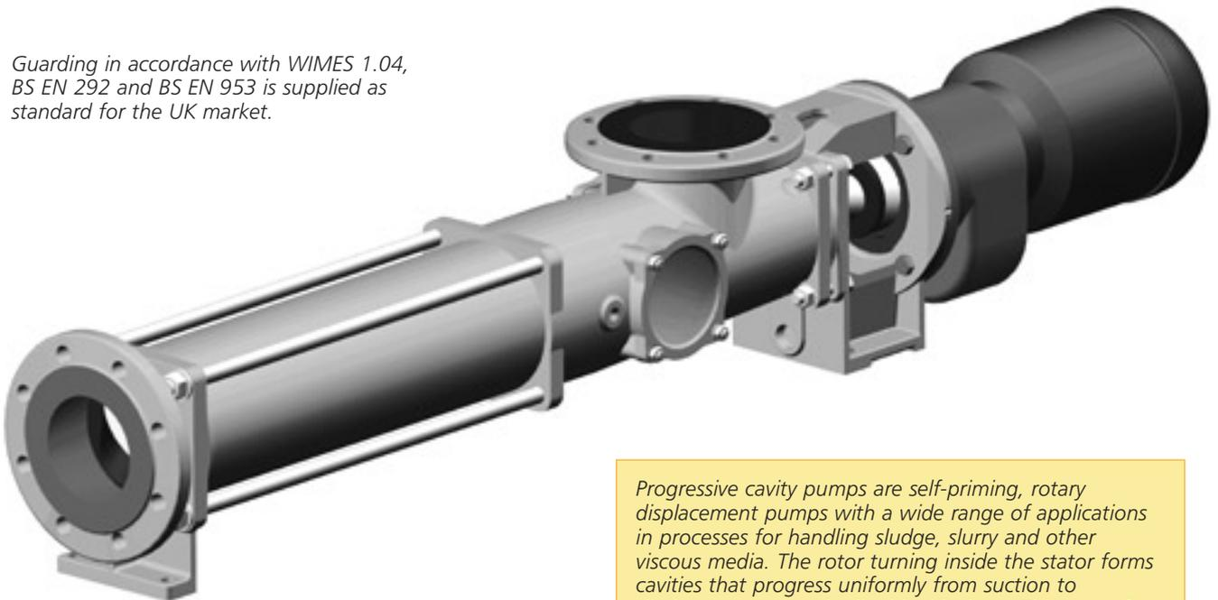
*Progressive cavity pumps are self-priming, rotary displacement pumps with a wide range of applications in processes for handling sludge, slurry and other viscous media. The rotor turning inside the stator forms cavities that progress uniformly from suction to discharge, carrying the liquid with them. This type of pump has the added advantages of providing highly accurate dosing.*
