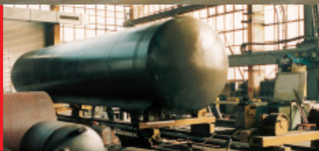
New epoxy coated tank.
