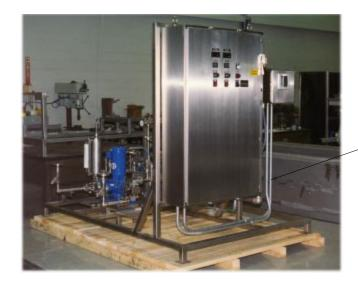
All stainless steel construction to minimize corrosion
