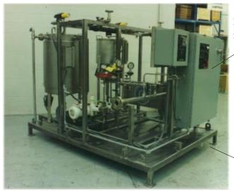
Electrical control cabinet with ratio and motor controller
