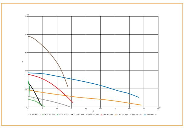
Flygt submersible dewatering pumps, 50 Hz
