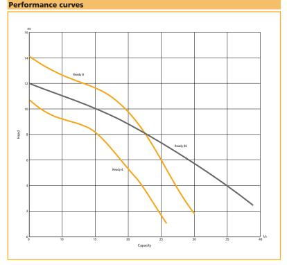
Flygt submersible dewatering pumps, 50 Hz
