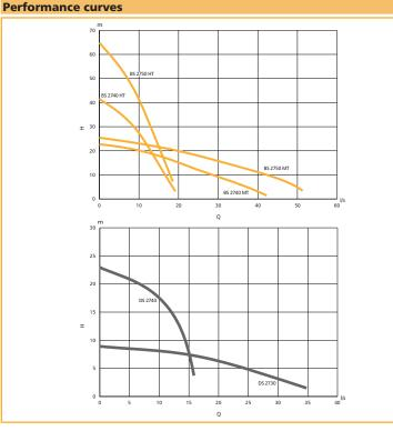
Flygt submersible dewatering pumps, 50 Hz
