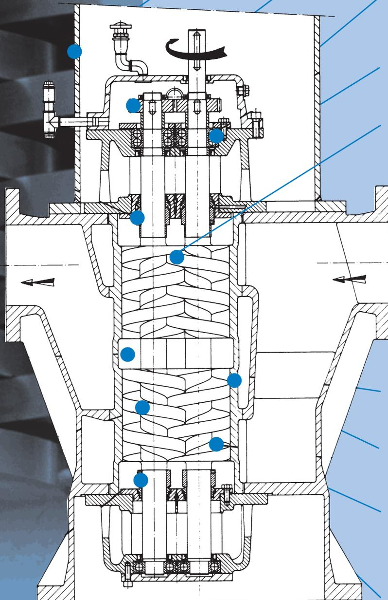
Drive by **commercial standard motors**, construction V1, all types of enclosure possible, therefore a motor bracket is optional.
